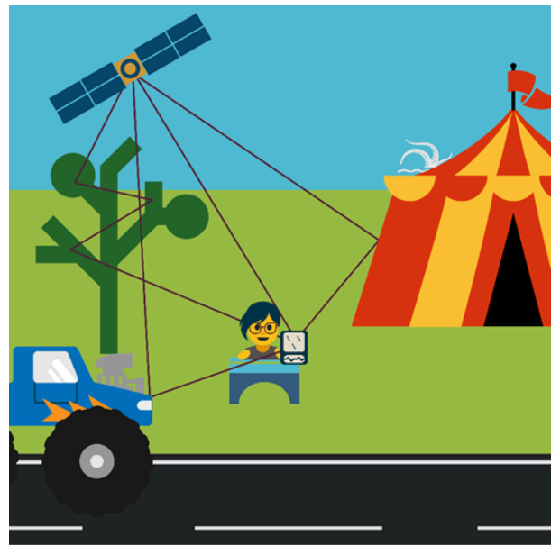
Figure 3.5(f): Multipath error
